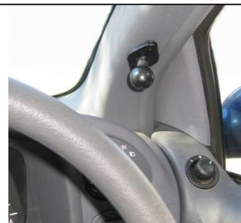
Fit the RAM mount extension arm loosely to the car column RAM base.
