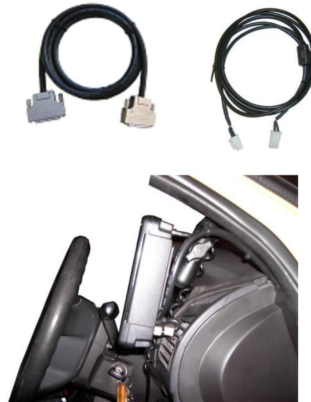
Connect the meter listening data cable. This runs from the junction box to the meter. If the meter is already connected to the EFTPOS terminal, disconnect the EFTPOS terminal at the meter end and re-connect using the connector on the meter listening cable. Connect to COM4 on the junction box.
