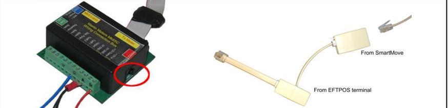
Connect the SmartMove terminal's RJ12 meter connection to the joiner on the Meter Listen Adapter
